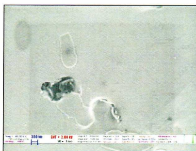
Fig. 15 SEM image of cracked BN inclusion in DC04 EK-B grade sample
