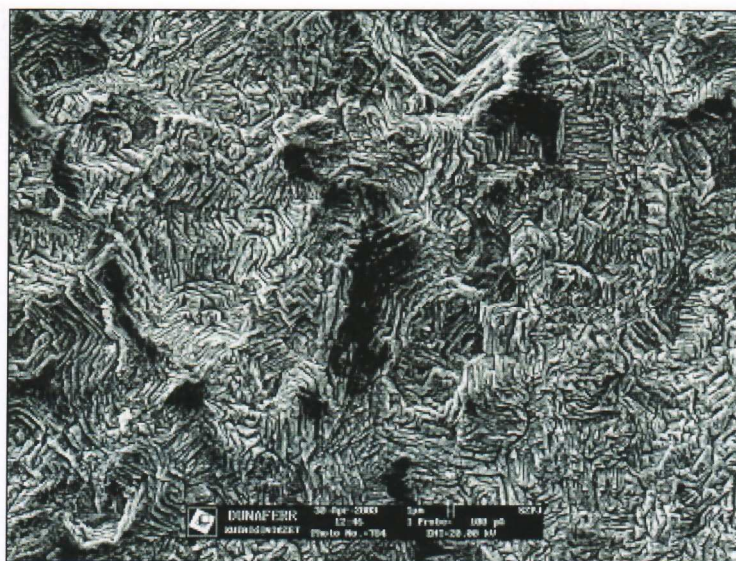
Fig. 7 The surface after pickling of the cold rolled DC04 EK grade specimens
