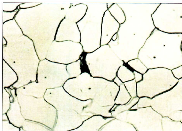
Fig. 11 The microstructure of hot rolled DC04 EK grade sample (nital, 500x)
