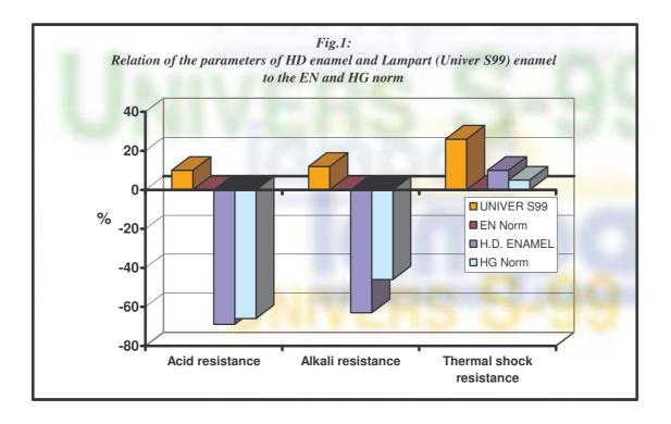
We can see, that HD enamel meets the requirements of HG and EN norm regarding the thermal shock resistance only. Its acid- and alkali-resistance are nearing the HG norm and are missed EN norm.
