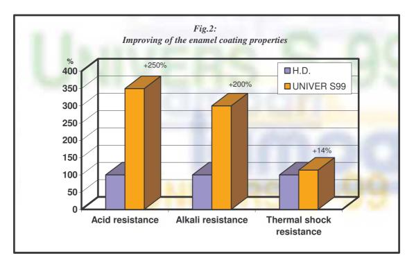
The acid resistance will improve by 250 per cent, the alkali resistance by 200 per cent, the thermal shock resistance by 14 per cent.
